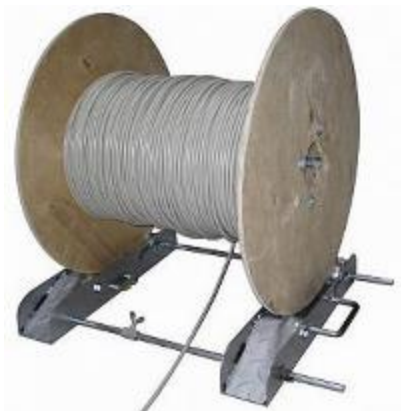
Figure 1. Example of an unwinder for a reel
