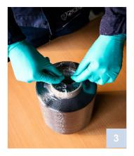
Pull the thermoretractable film along the welding **(3)**
